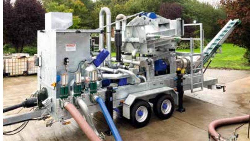
The medium is drawn from the large slurry container into the V2S separator. Mechanical separation of the aqueous phase from the solid and suspended matter takes place here. The V2S separator is positioned on a tandem-axle trailer licensed in line with German road traffic regulations. A key feature is the combination of mechanical screening technology and vacuum. A patent application has been submitted for this centrepiece.
